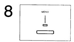
After programming all the numbers, press the MENU button to end the operation.
